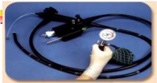
Perform Leak Test again before disinfection.
